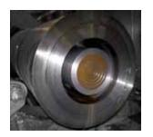
Trepan operations can be applied to efficiently meet needs of customers. The most basic service provided is a rough hole through a bar's entire length. In some cases, it is desirable to drill from both ends. It is possible to create a stepped bore by drilling a different sized hole from the opposite end. If a hole does not go through, it
