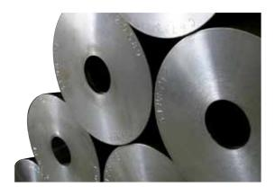
It is possible to apply trepanning in holes over a great range of sizes, but with few exceptions trepanning is generally applied in a range of 4.1" to 15.75". Below that range, solid drilling with BTA single tube system is optimum from 1". The smallest holes generally require gundrilling. Above 15.75", rough and finish boring operations are available often reaming from a smaller
